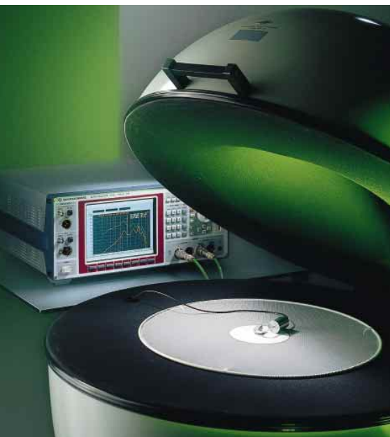
FIG 1 Measurement of coherence and transfer function on hearing aid using Audio Analyzer UPL Photo 42 642
