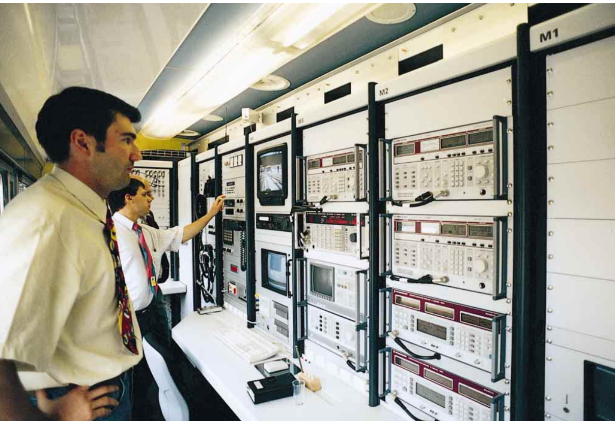
FIG 2 Interior view of measurement carriage with test receivers, modulation analyzers and monitors Photo: Roschi Telecommunication AG
