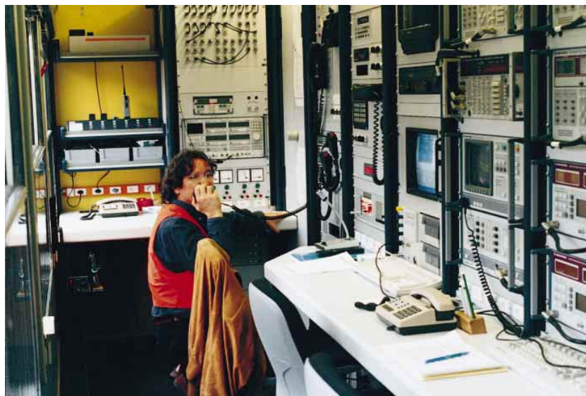
FIG 3 Onboard equipment includes radio coverage measurement instruments as well as Radiocommunication Tester CMT54 (background) Photo: Rockrohr
